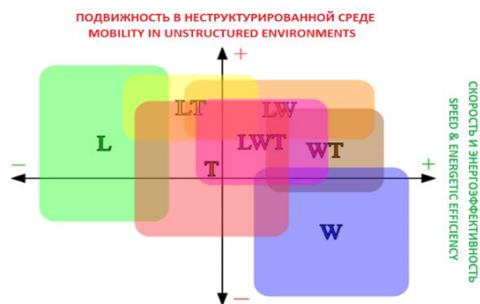
Figure 1. Mobility in unstructured environments vs. speed and energetic efficiency of the possible hybrid locomotion systems (Adapted with permission from [13], copyright 2012, L. Bruzzone and G. Quaglia).
